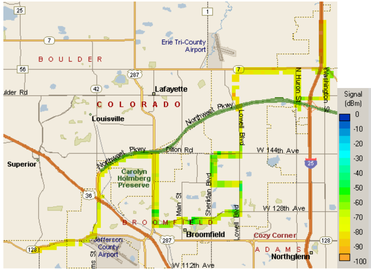
Figure C-2. Signal Strengths of Existing Access Points along the Test Route.
