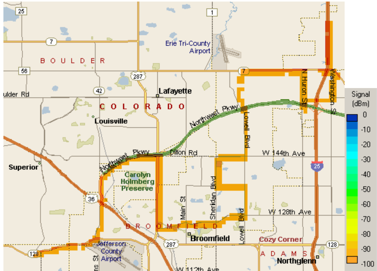
Figure C-3. Average Noise along the Test Route.
